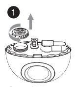
Remove the screw cap.
