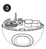
Note: Make sure the screw cap is tightened.
