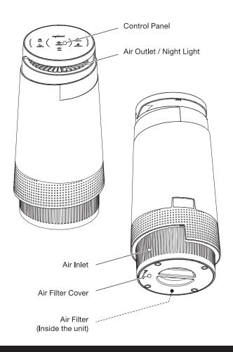
WARNING: The plastic bag around the filter must be removed before use.
